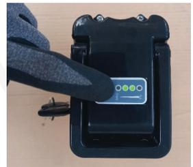
press of the red button: 4 led 100% charge, 3 led 65%, 2 led 35%, 1 led 10%.
